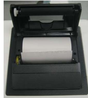
**Figure 1.5.3-2 Printer paper compartment lid open**
