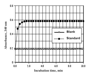
**Figure 1.** Increase in absorbance at 340 nm on incubation of 20  $\mu$ g of D-malic acid with hexokinase and glucose 6-phosphate dehydrogenase in the presence of NAD<sup>+</sup>.
